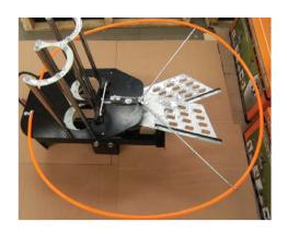
Rotate arm counter clockwise to 12:00. Insert Black Main Spring into silver swiveling spring hook.
