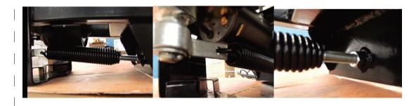
Because the clay lands directly onto the throwing arm, the White Wing needs little adjustment. Loosen the two bolts on either side of the trap to adjust your throwing angle. Once desired angle is reached, tighten bolts back.
