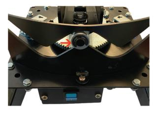
NOTE: For easy re-installation, set the middle screw first. Make sure all screws are in prior to tightening completely.
